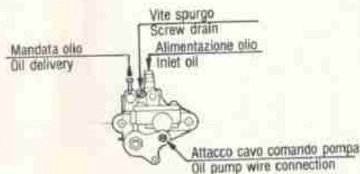
FIG. 24 Pompa olio Oil pump
