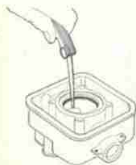
FIG. 31 Controllo segmenti Piston ring check
